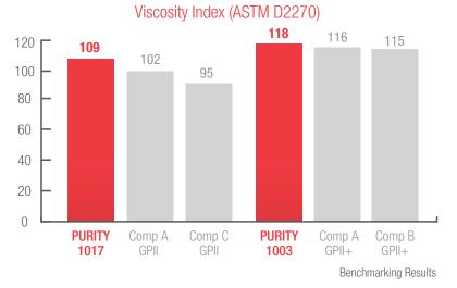
High VI oils are preferred for service in which a constant viscosity is desired under conditions of varying temperature. Viscosity stability contributes to greater fuel efficiency in motor oils and reduced power consumption in industrial lubricants.
